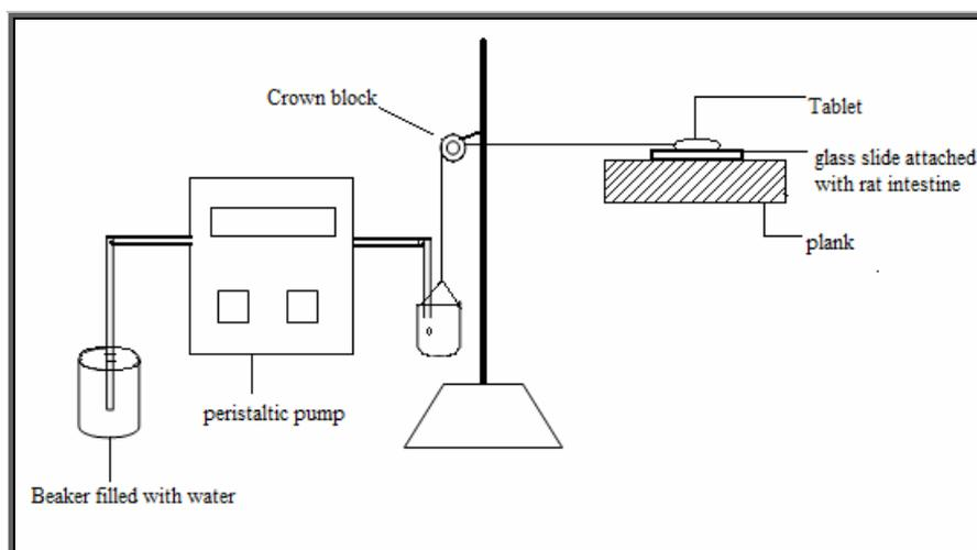
Figure-1: The scheme of the device used in the mucoadhesion study
