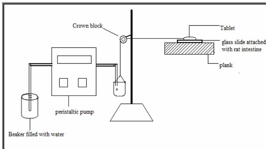
Figure-1: The scheme of the device used in the mucoadhesion studie
